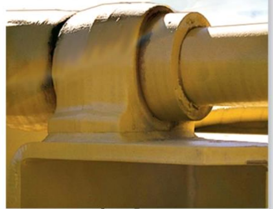
This thrust bearing is used to support the drive shaft on a machine. (7)
