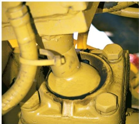
This ball-and-socket joint provides a connection for the housing of an earth grader to its frame. (4)
